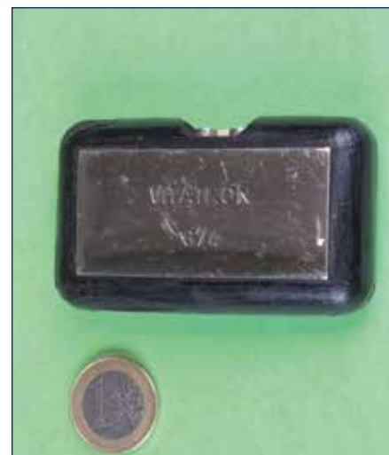
Fig. 2 V34036 - MIP-100 - 'Groningen' pacemaker, fixed, dual heart rate, 1965 onwards, single (-) lead / (+) plate.
