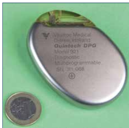
Fig. 6 V33076 - Quintech DPG - diagnostic pulse generator; world's first microprocessor based pacemaker (model 921), 1981 onwards.
