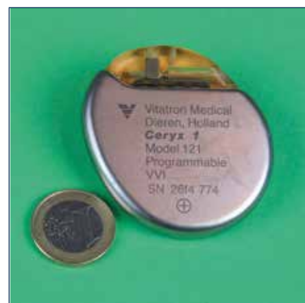
Fig. 9 V33085 - Ceryx 1 , single chamber VVI multi-programmable pacemaker, model 121, 1983.
