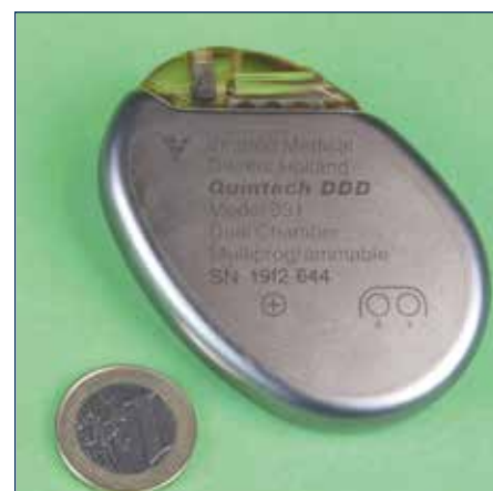
Fig. 8 V32995 - Quintech DDD , first dual chamber / dual lead pacemaker with automatic arrhythmia detection, model 931, 1984 onwards.
