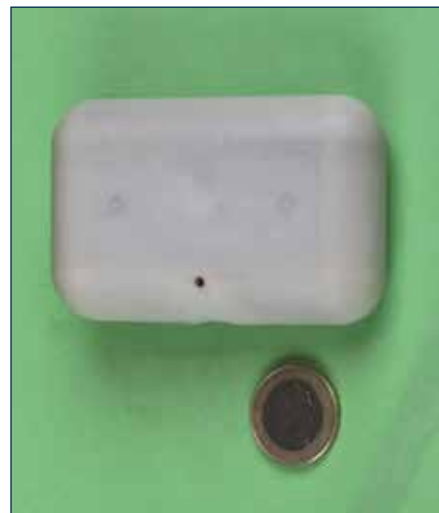
Fig. 1 V34040 - Early series Vitatron pacemaker PM 100, 1963 - 1965, fully sealed, 2 leads. Please note the one Euro coin is for size reference only.
